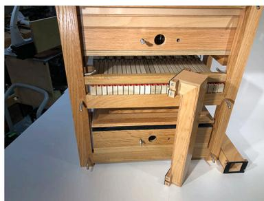
Find the straight wind channel that connects the reservoir to the wind chest above.
