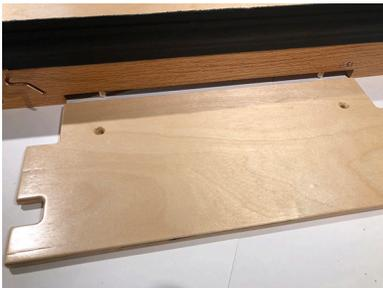
Two pins on the bottom of the bellows fit into those hole.
