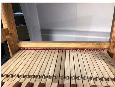
Slide the small crossbar onto the tall pins, tapered side down. Don't forget to match the numbers!
