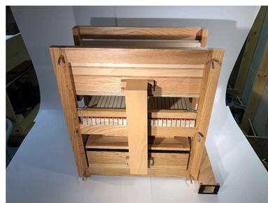
Slide the wind channel onto the thumbscrews and add the other thumbscrews, snug, but not too tight.
