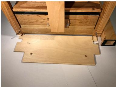
The other side of the plate has notches for the legs of the frame.
