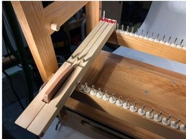
Each key slides onto a metal pin at the top and bottom
